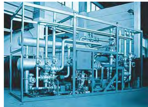
Dual secondary control circuit for temperature control of a plastic machine.
